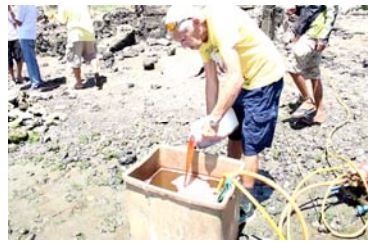
OSE II being added to the natural sea water in the mixing tank
