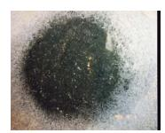
It was determined that 0.25 inches, or ¼ of an inch of grease remained on the surface. This represents a 92.2% reduction of grease by volume. The TRA lab confirmed the OSEI Grease reduction findings tests as well.
