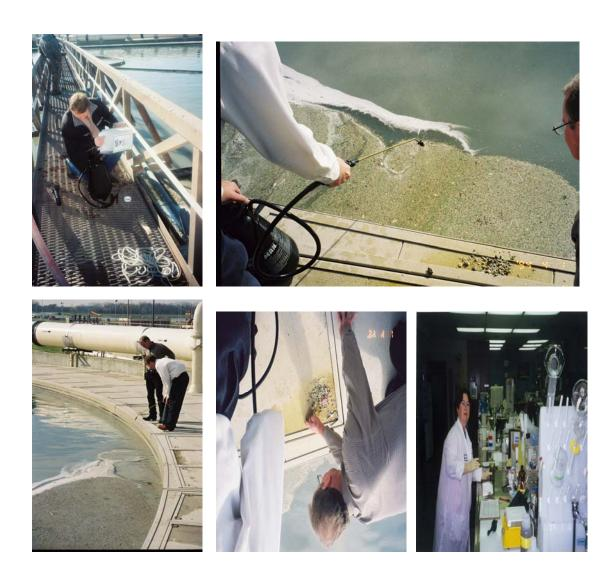
After application of OSE II, TRA personnel removed some of the oil and grease to see how the initial reactions of OSE II were affecting the breakdown of the oil and grease. A subsequent sample was extracted 4 hours after OSE II application by TRA. This retention pond test showed OSE II reducing the size of the oil and grease globuals, as well as the measurable volume of the oil and grease. As OSE II breaks down the oil and grease, the globuals became smaller and smaller, since OSE II
