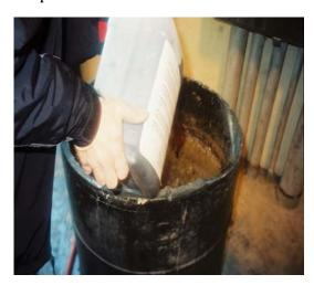
Next 26 ounces of OSE II was applied to the grease in the drum. The aeration device was turned on and 2 samples of grease were extracted for analysis.
