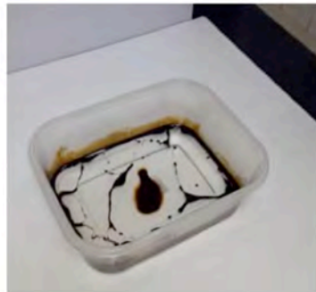
Photo No. 9 immediate dispersal of traces of crude oil to the vessel walls
