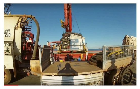
The truck on the left, extracts or sucks up the effluent contaminant, the truck on the left has OSE II and water mixture to apply to the contaminant fuel/hydrocarbons. You may have to mix OSE II and water in the truck more than one time depending on the amount of contaminant/ fuel/hydrocarbons.
