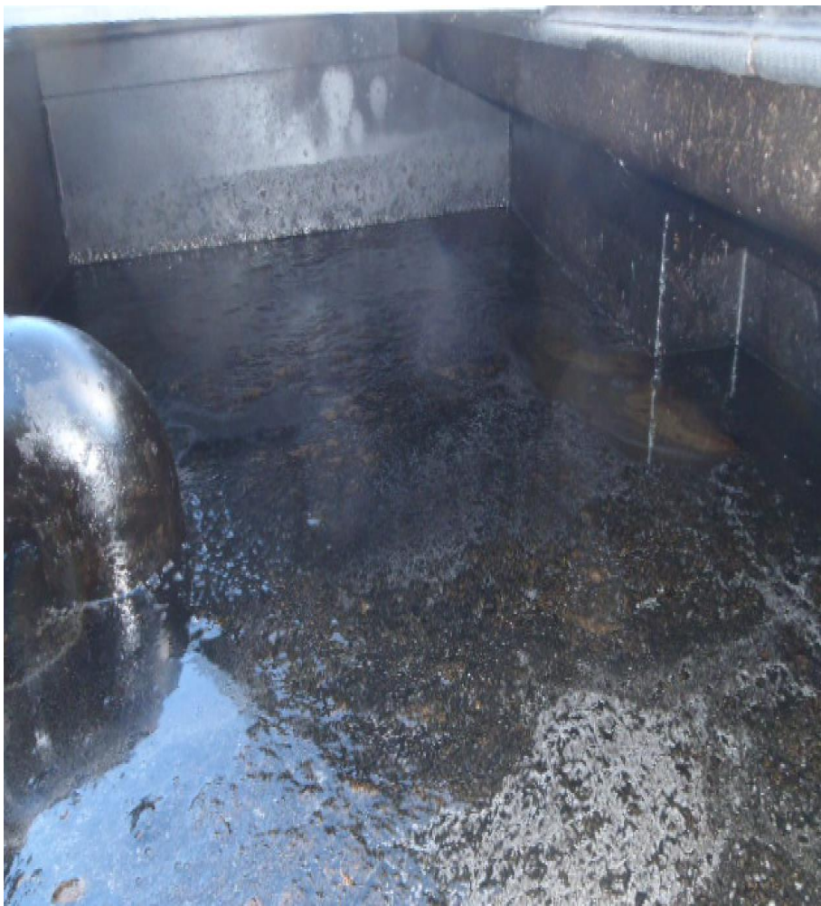
Once OSE II started reducing the adhesion properties of the oil and causing it to lift, allot of oil started being pulled into the metal container, where the oil volume could be monitored
