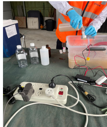
Mixing OSE II to apply to the PFAS Contaminated water
