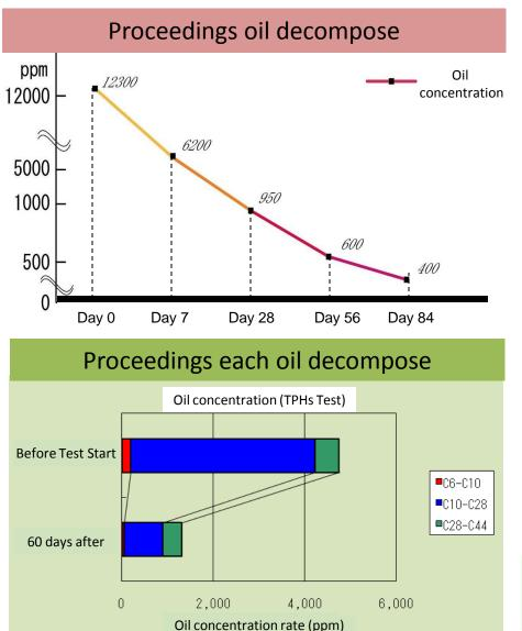
About ppm (parts per million) : ppm is rate of contamination level of each soil. We multiply amount of soil by ppm. For Example: If the rate is 12300ppm from amount of 3000kg soil which means contain oil about 37kg (1.23%). \*Usually most of pollution rate is 1000-7000ppm.
